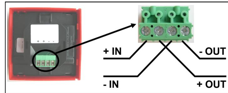
Picture 7 - front device's wiring to the loop
